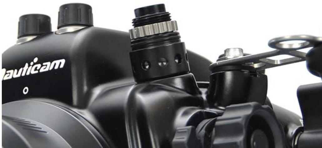
LED turns from the slow flashing blue to solid green indicated the housing is sealed and ready to use. A dual activation valve which accepts the low pressure BCD inflator hose quick disconnect is also available. This uses tank pressure to create a venturi effect to pull the vacuum. Be aware that not all BCD inflator hoses are the same size so check the size compatibility before ordering this valve.
