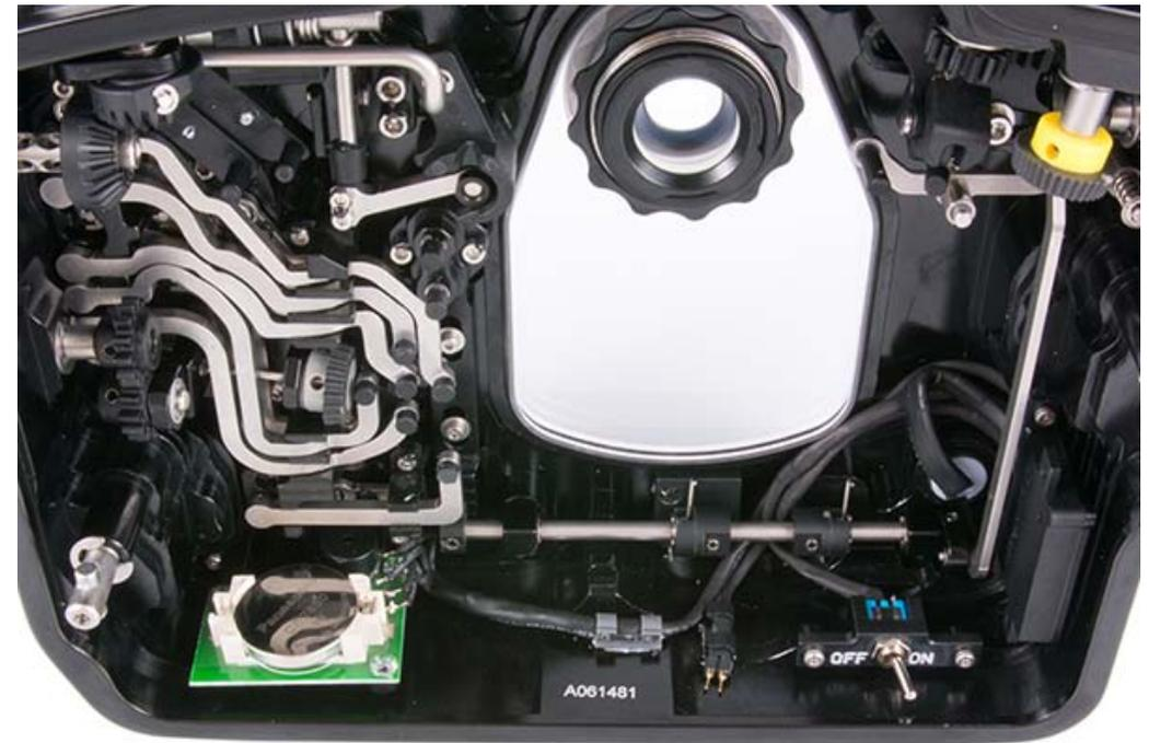
valve and a simple light weight pump. The electronic monitoring circuitry looks very much like the leak detection circuitry which has come in all of the past Nauticam housings. The new vacuum system uses the same type of warning light and audible alarm found in all current Nauticam housings. The noticeable difference is the new on and off switch now located inside the housing.
